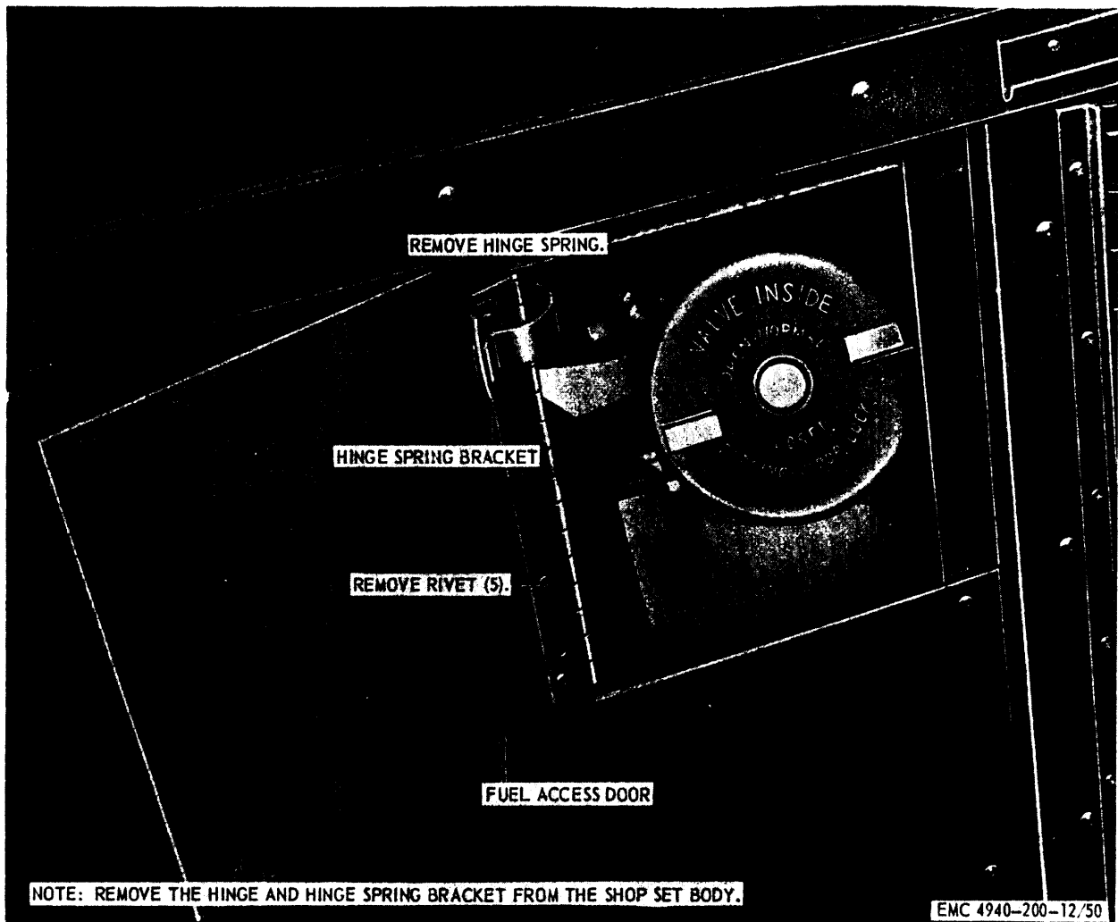
Figure 62. Fuel access door, removal and installation.
